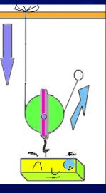
The mechanical advantage of a moveable pulley is equal to the number of ropes that support the moveable pulley.
