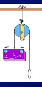
A fixed pulley changes the direction of a force; however, it does not create a mechanical advantage.
