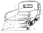
A ramp is used for loading this truck. A mover can pull a cart with a heavy object up the ramp. This is much easier than lifting heavy objects into the truck.
