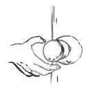
When you turn the large knob on a door, a rod on the inside releases the a latch that holds the door closed. It would be difficult to turn the rod, if the knob wasn't attached to it.
