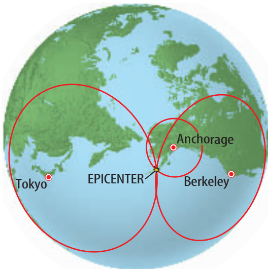
Figure 6 After distances from at least three seismograph stations are determined, they are plotted as circles with radii equal to these distances on a map. The epicenter is the point at which the circles intersect.
